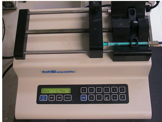
Figure 3.8: Electronic syringe pump used to eject and control the flow rate of the liquid polymer.
