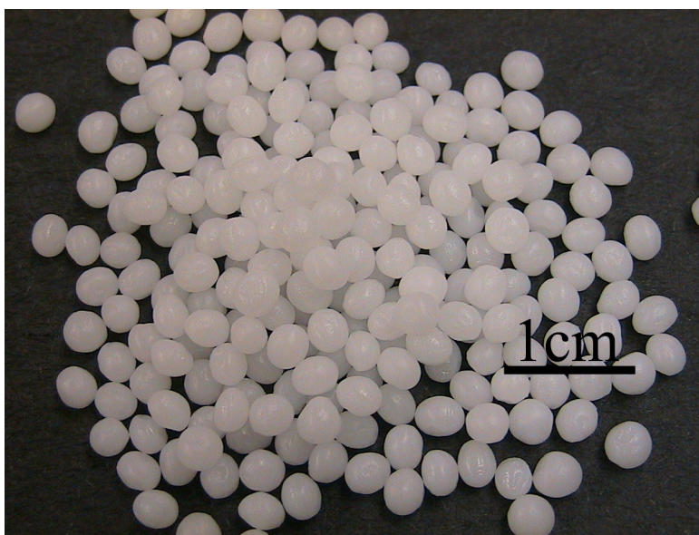
Figure 3.12: Polycaprolactone (PCL) with M_w 42,500 in pellet form.
