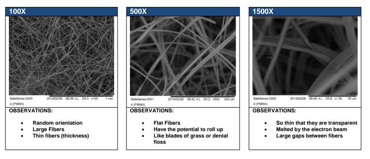
Specimen 1 A (PMMA), Point 2
